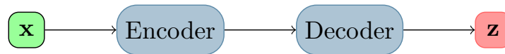
Figure 2.8: Encoder-Decoder architecture. Each *coder sub-networks is made of one or more RNNs composed by one or more RNN layers.
